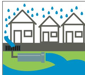
As our City grows, natural areas are covered by hard surfaces that do not allow rain to soak into the ground. Underground pipes and catch basins, along with stormwater facilities, are built to prevent flooding and filter pollutants from stormwater.
