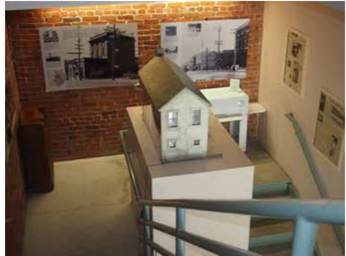
▲ Figure 8: The stairwell between the first and second floors of the museum. There are three large collection objects exhibited in this space with no barriers to prevent touching. The two placed on the pathway are also obstacles to safe egress from the building in the event of an emergency.
