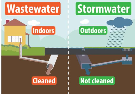
Springfield's stormwater system is separate from the wastewater system. **Wastewater** collects used water indoors and it flows to the regional wastewater treatment plant for cleaning. Then it's released into the Willamette River.
