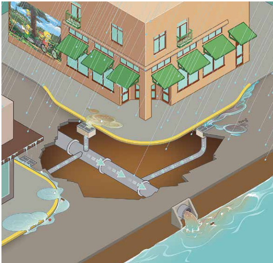
Apply carefully because de-icers wash into the stormwater system. That water isn't cleaned before it enters local waterways.
